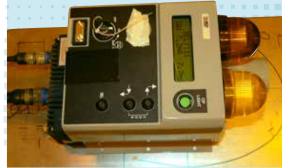
Qualification of radioprotection beacons performed in the irradiator PAGURE (MIRION Technologies)
