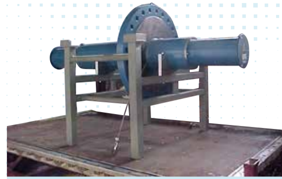
Ageing irradiation performed in the CALINE cell on a HTA electrical penetration (Auxitrol - EDF/Septen)
