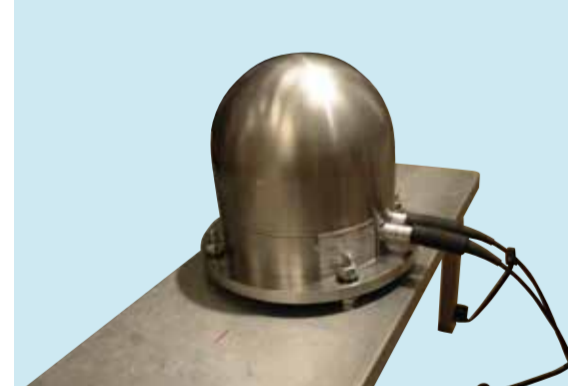
Qualification of radioprotection beacons performed in the irradiator POSEIDON (MIRION Technologies)
