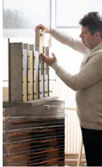
Paint coating materials qualification performed in the accelerator VULCAIN (EDF/CEMETE)
