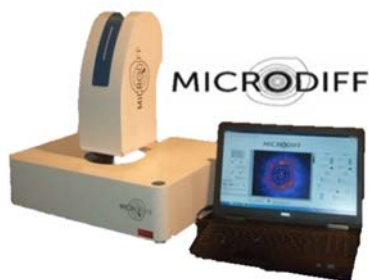
Fig. 1. Photograph of the integrated MICRODIFF instrument for fast and accurate identification of clinical pathogens using elastic forward scattering
