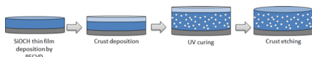
Figure 1: Schematic representation of the process proposed to obtain the foaming of SiOCH thin films.
