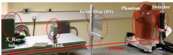
Fig.1. Schema of the experimental system including a spectrometric detector (32 energy bins).
