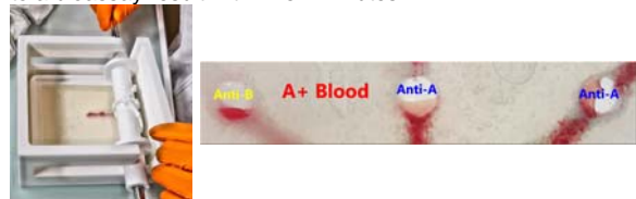
Figure 2: Blood typing prototype for effective identification of the blood type of a whole blood sample.
