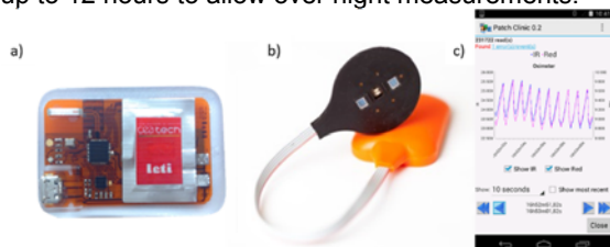
Figure 1: a) Patch, b) SpO 2 sensor and c) smartphone application.
