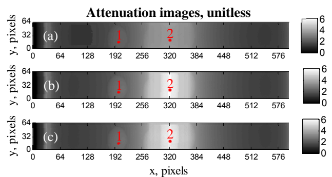
Figure 1: Total (a), primary (b) and corrected total (c) attenuation images. Control points for spectra displayed in Figure are indicated with numbers on the attenuation images.
