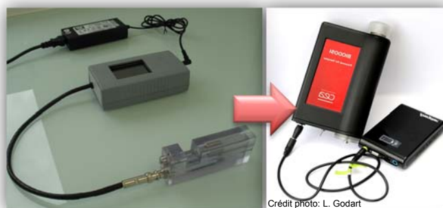
Figure 2: Evolution of the electrostatic precipitator from a simple experimental device to a robust prototype (from Roux et al. [3]).
